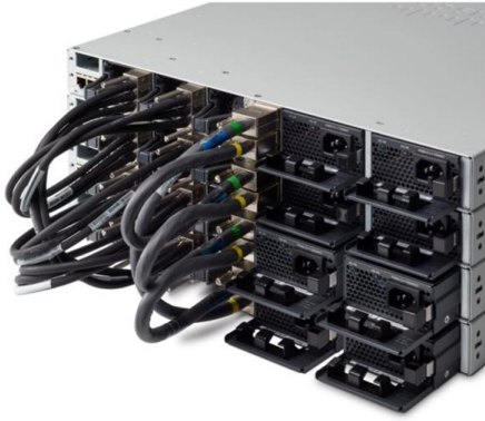
Figure 7. Cisco Catalyst 9300 Series StackPower
